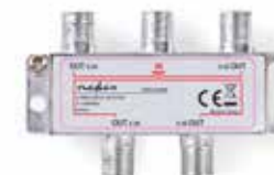
CATV Splitter • 5 - 1000 MHz • Insertion loss: 8.0 dB • Number of Outputs: 4
