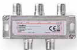
Satellite Splitter • 5 - 2400 MHz • 11.5 dB • Number of Outputs: 4
